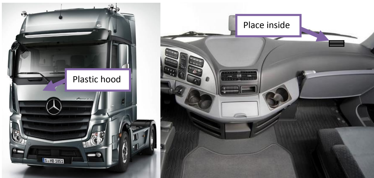
Figure 47.1 Possible mounting places in trucks
